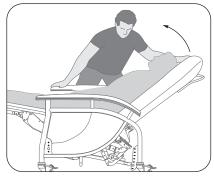
2. The caregiver squats with their back straight and pushes down on the center of the leg rest to lower it down and store it under the seat.
