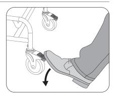
WARNING: BEFORE HANDLING OR MAKING ADJUSTMENTS, ALL 3 BRAKES MUST BE APPLIED AS SOON AS THE CHAIR IS NOT USED FOR MOVING SO THAT IT REMAINS STABLE.
