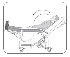
2. To close the leg rest, apply downward pressure with your legs on the leg rest. Pull lightly on the end of the armrest simultaneously with your hands so that the footrest is placed under the seat.
