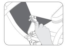
Tighten or loosen the pressure bolt behind the backrest support (one on each side) depending on the angle desired.
