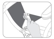
4. Tighten the locking nuts on each side that had been loosened.
