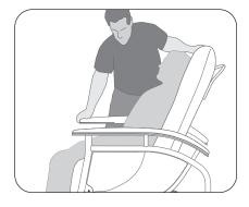
The caregiver then pushes back on the backrest with one hand while the other hand leans on the armrest while transferring their weight from one leg to the other. This maneuver will cause the backrest to tilt backwards while rising the leg rest simultaneously.
