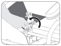
To adjust the backrest angle, loosen the locking nuts (one on each side).
