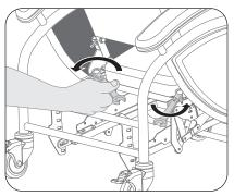
Adjust the depth correctly by moving the backrest on the seat slides and re-tighten the bolts. Adjust both sides to the same depth.
