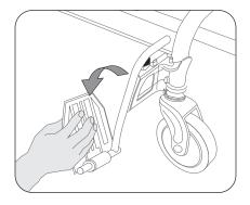
4. To store the footrest, raise the footrest upward, activate the black lever and pivot the footrest outward until it locks into place.
