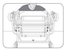
2. Using a <sup>1</sup>/<sub>2</sub>" (13 mm) wrench, remove the 4 bolts (2 per side) that hold the seat support.
