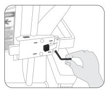
Adjust the trunk support to the desired position.
