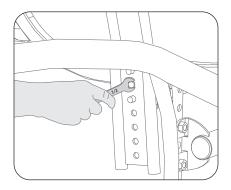
Position the armrest at the desired height and replace the bolt, without forgetting the flat washer and the lock washer.
