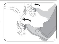
WARNING: NEVER MOVE THE CHAIR WHEN THE BRAKES ARE APPLIED. THIS COULD RESULT IN BREAKAGE, INJURY OR DEATH.
