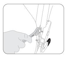
3. Position the lateral supports at the desired height. Retighten the nuts.
