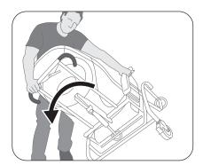
3. Under the seat behind the chair, find the series of 4 holes in an arc pattern that control the backrest angle. Using a 1/2" (13 mm) wrench, remove the bolts on each side.
